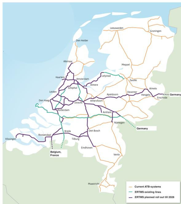
Figure 1. Planned ERTMS roll out in The Netherlands from 2024-2028 (translated from: [www.ertms-nl.nl](http://www.ertms-nl.nl), Retrieved August 16, 2017)
