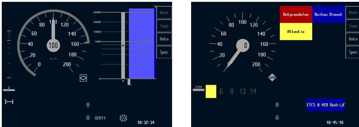
Figure 3. DMI ETCS in SLT trains during ERTMS pilot. Left: ETCS level 2. Right: STM ATB.
